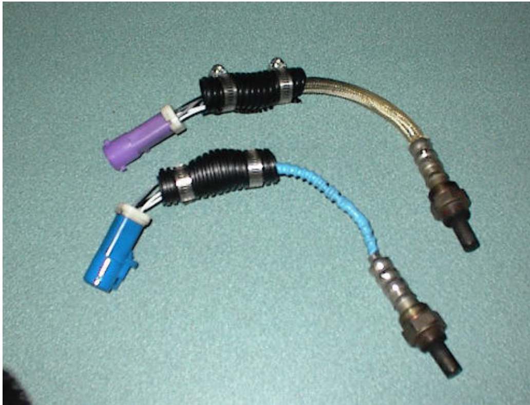
Fig. 3 Completed modified O2 sensors ready for re-installation into the vehicle
